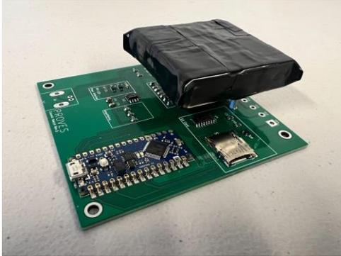
**Figure 5: Cosmic Watch with Arduino Nano Every**
