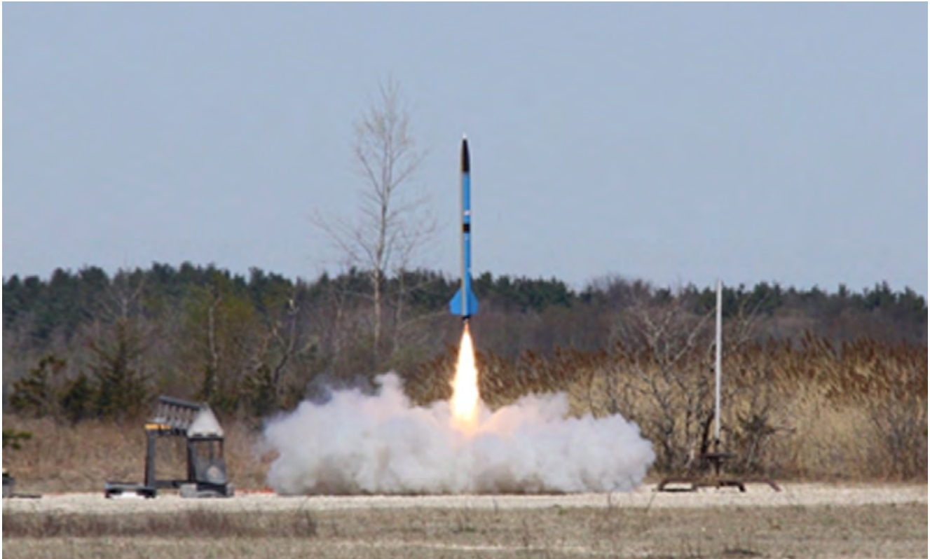
Figure 3 – The Spacehawks rocket was a Wildman 4” Drago, shown launching here on an Aero-tech K550. The rocket had small payloads in the avionics bay, the nosecone, and in the tiny space between the motor and body tubes.
