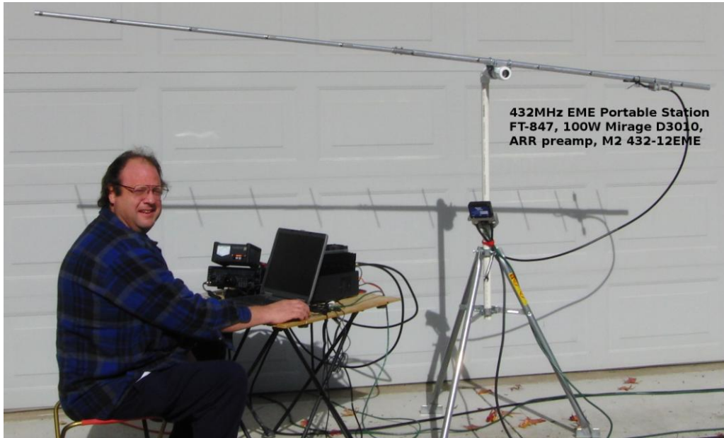
K6CLS with rig and 12 el yagi use on 70 cm EME
