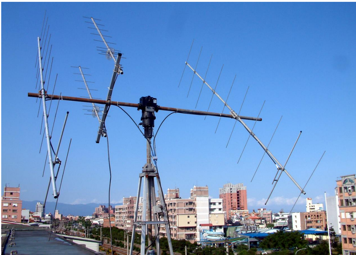
BX1AD 2 yagi array used on 70 cm EME
