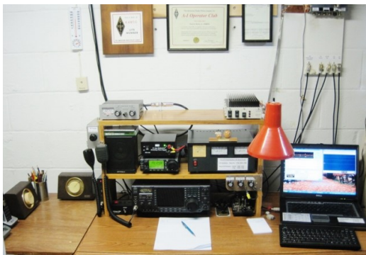
The main station layout at K4MSG showing the HF and VHF/UHF equipment and laptop computer, *minus* the 144 MHz amplifier (which usually sits on the top shelf next to the 432 MHz amplifier).
