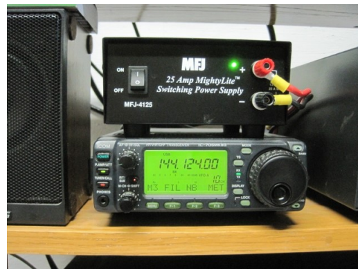
Close-up of the IC-706MkIIIG transceiver and MFJ 25-amp switching power supply.
